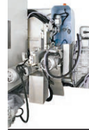
3 Mandrino per gocciolatoio e mandrino multifunzione. Water drip unit and multifunctional spindle in horizontal position.
