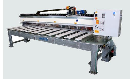
Miter saw for 45 degree cutting
