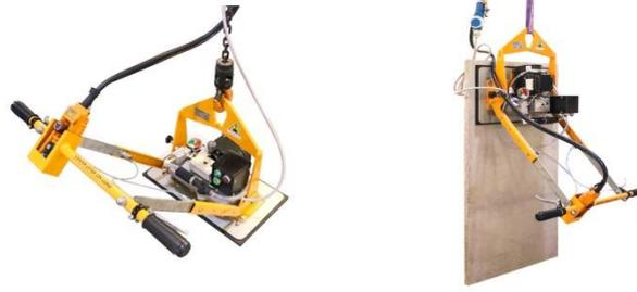
Featuring a sliding valve, the AEVL1-250 is a powered vacuum lifter which is suitable for securely handling small-sized materials. By means of a vacuum tank, the lifter ensures safe pick-up in the event of a sudden power break to the vacuum pump.
