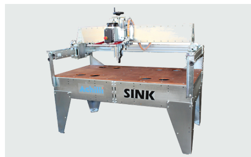
SINK machine for sink cut-outs
