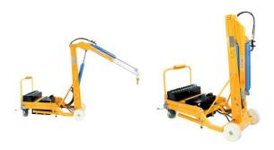
The Powered Counterbalance Crane with Lateral Movement has an adjustable boom to allow for maximum adjustment and versatility to lift a variety of loads. The boom is raised via a 12V battery-powered hydraulic pump. The boom also telescopes out for greater reach. The counterbalance design eliminates the need for front legs. This makes the unit easier to manoeuver and allows the crane to reach tight, hard to reach areas.
